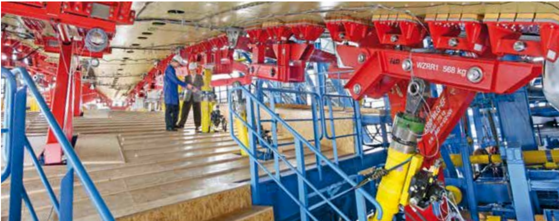
4 | Hydraulic cylinders are also used for systematic application of stress to the hull
