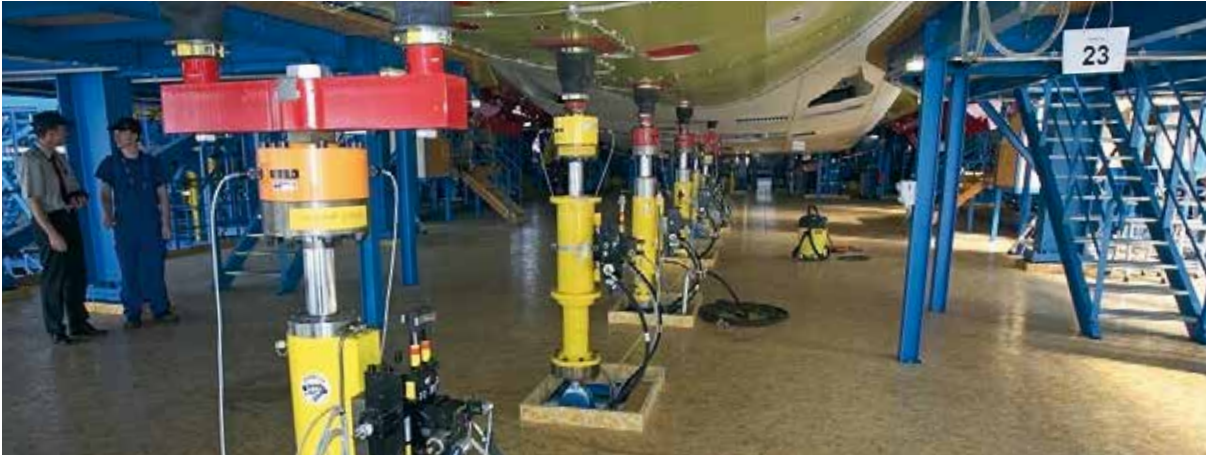
5 | Application of stress to the hull using hydraulic cylinders.
